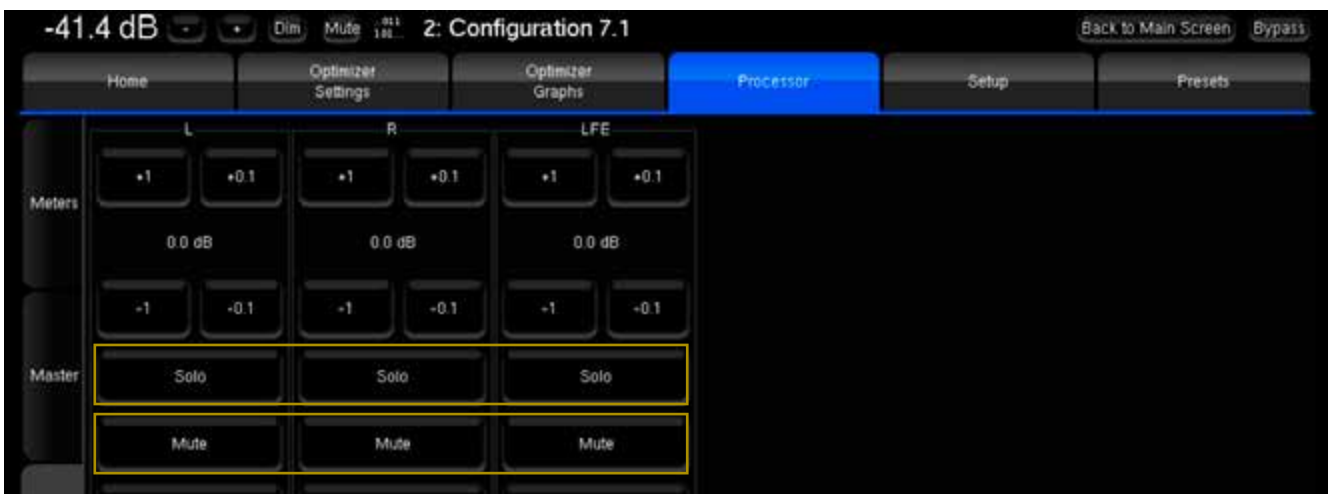
Figure 97: Mute and Solo buttons in the Inputs page of the Processor menu
