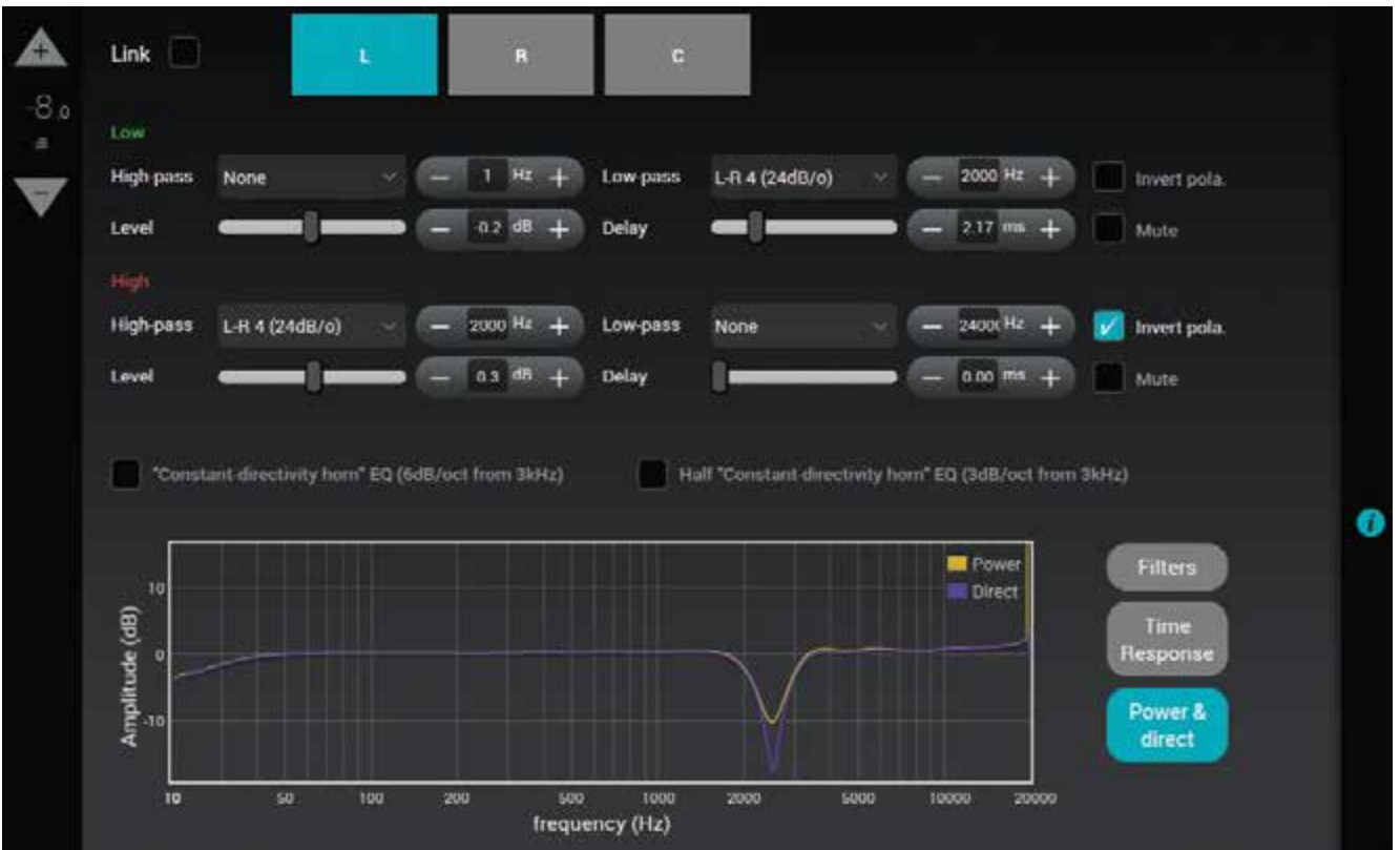
Figure 79: frequency response (power and direct)
