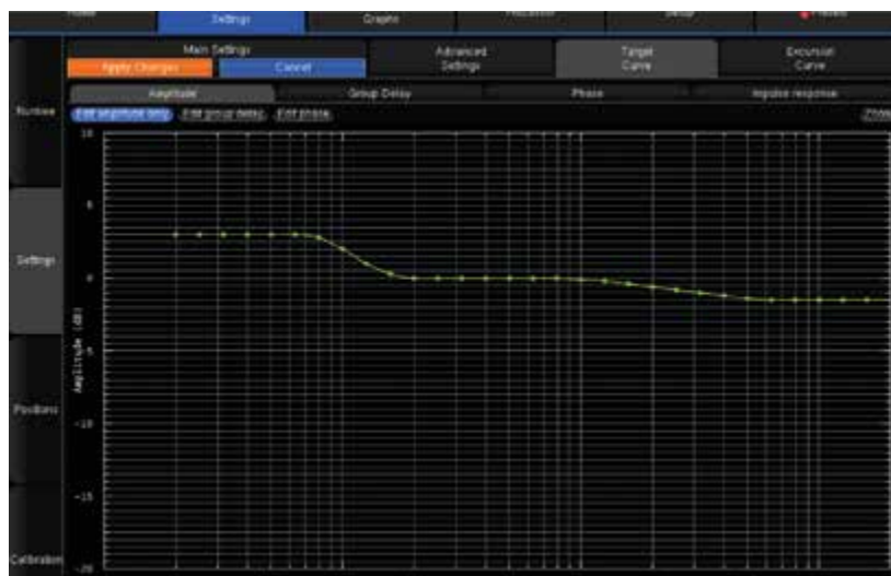
Figure 111: Example of a Target Curve in the Advanced Settings user interface
