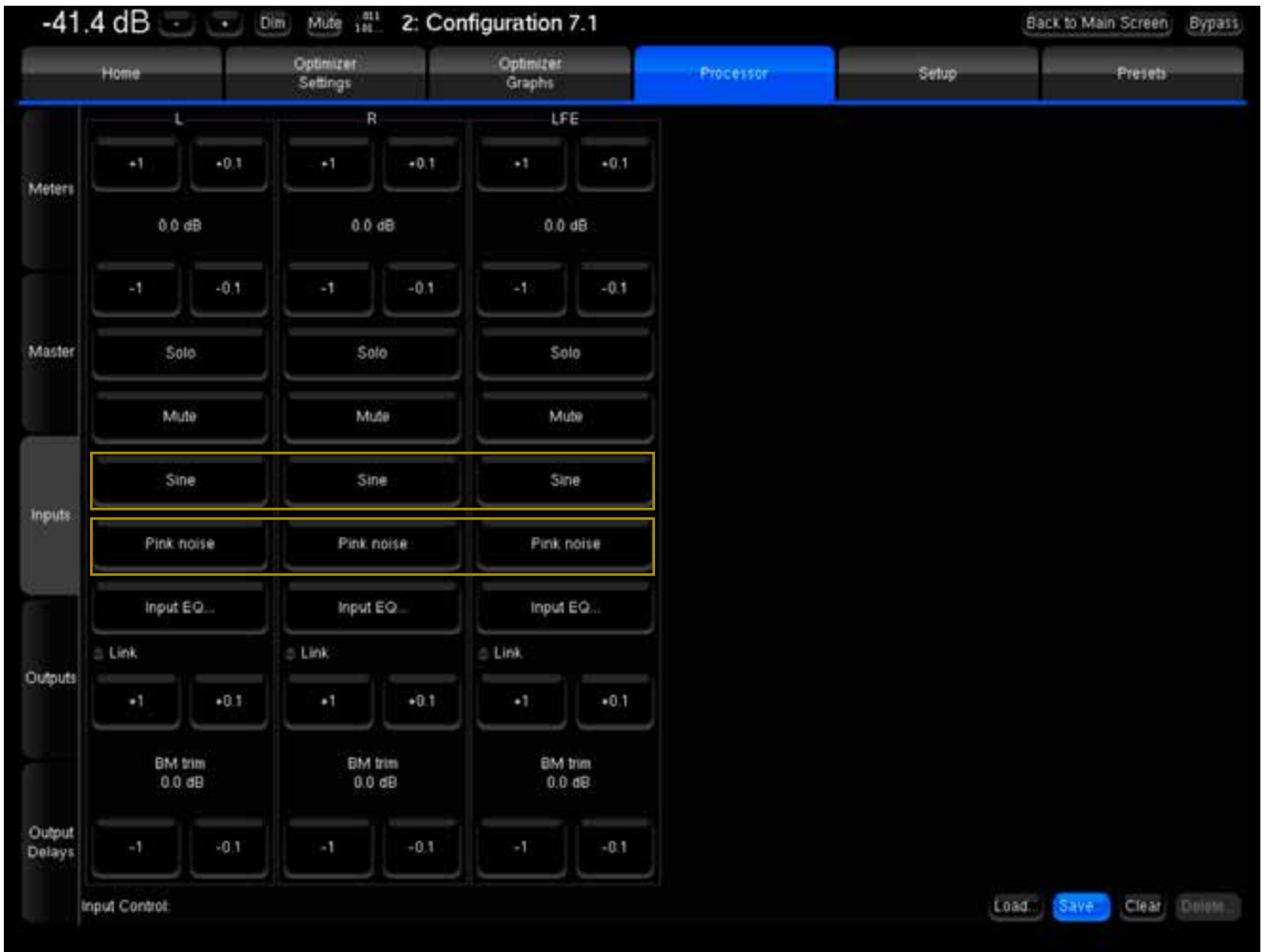
Figure 96: Sine and Pink Noise buttons in the Inputs page of the Processor menu
