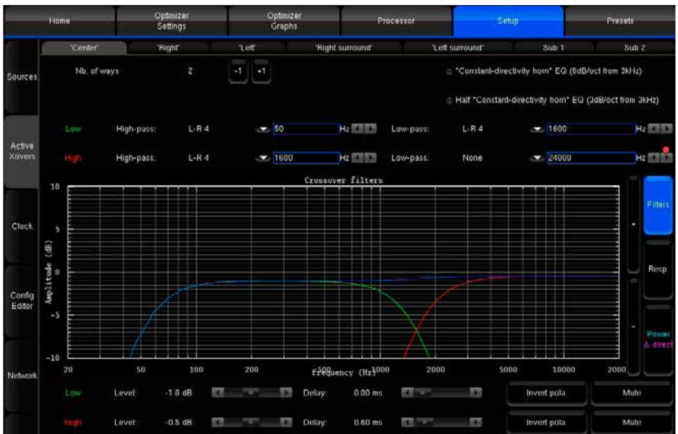
Figure 127: Performing the calibration of the active crossovers
