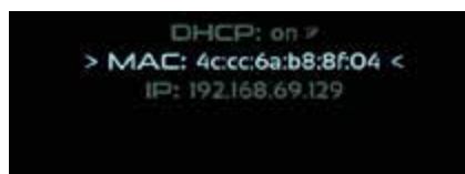
Figure 21: IP address in the Setup > Network > Ethernet page via the front panel
